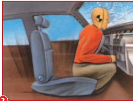
2 When the driver hits the brakes, the car stops. If the stop is sudden and the driver is not wearing a seat belt, the driver keeps moving forward.
