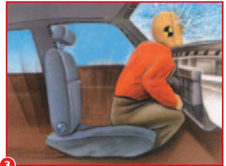
3 Finally, the windshield applies an unbalanced force that stops the driver's forward motion.
